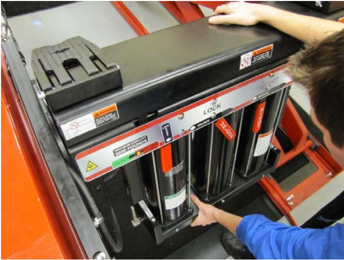
Pivot lock indicator in the "LOCKED" position.
