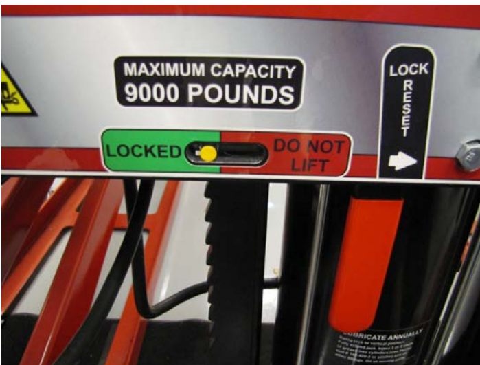
Pivot lock indicator in the "LOCKED" position.
