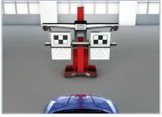
Calibrate vehicle forward facing camera to target
