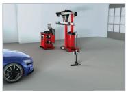
Calibrate vehicle forward facing radar to reflector
