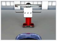
Calibrate vehicle forward facing camera to target
