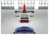
Calibrate vehicle forward facing camera to target
