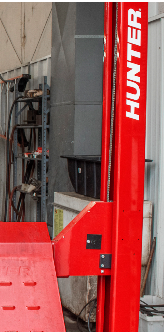
20-3145-1 – 17.5" Ramp Extension Kit (for low-clearance vehicles)
