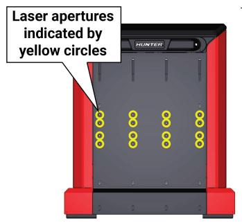
The Class 3R laser apertures are located at the front faces.
