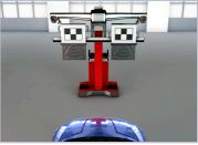
Calibrate vehicle forward facing camera to target
