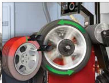
The Road Force® Elite's diagnostic load roller detects high spots in the tire and rim.
