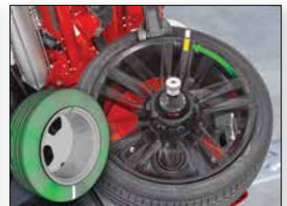
The tire changer dual rollers hold the tire in place to match the stiffest point on the tire to the lowest point on the rim.
