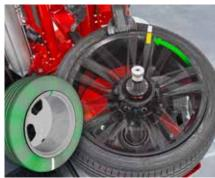
By combining tire changer bead massage with Road Force® match-mounting, virtually all vibrations can be eliminated.
