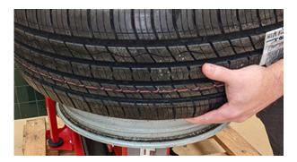
Raise the lower roller until the lower bead is slightly above the rim, then indent the roller. Rotate wheel until the entire bead is lifted from the rim. Remove tire from rim.
