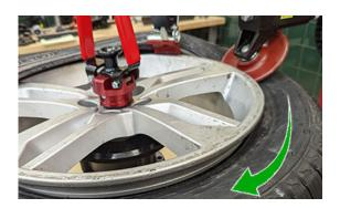
Rotate **slowly** while keeping the top bead in the drop center. For challenging tires or partially seated bead, use the bead press to help.
