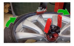
6 Rotate while pressing down on the tire with the upper roller.
