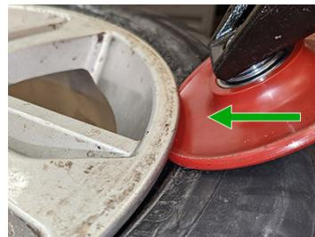
3 Rotate wheel. Apply lubrication while rotating wheel and pushing the bead off the rim with the bead roller
