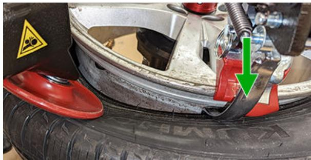
With the upper roller pressing down on the tire, bring your tool head down insert in between the bead and the rim, rotate tire while doing so to ease tension.
