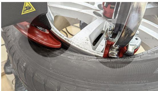
6 Rotate while pressing down on the tire with the upper roller.
