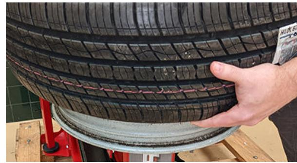
6 Raise the lower roller until the lower bead is slightly above the rim, then indent the roller. Rotate wheel until the entire bead is lifted from the rim. Remove tire from rim.
