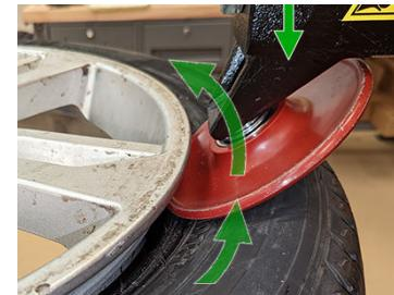
4 Stop when bead is removed from bead seat. Move upper roller out of the way.
