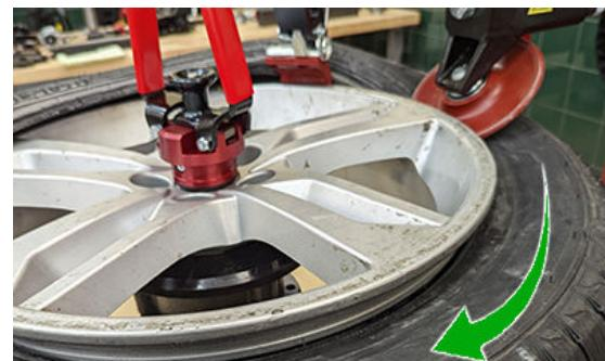
7 Rotate **slowly** while keeping the top bead in the drop center. For challenging tires or partially seated bead, use the bead press to help.
