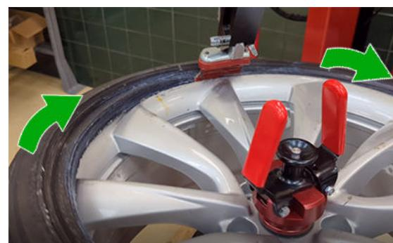
5 Lower the upper roller arm on the tire and indent right underneath the rim as shown.
