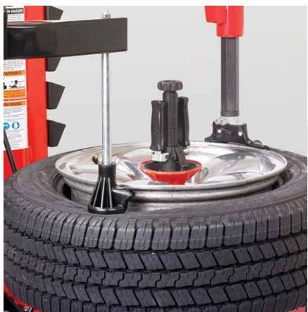
Press arm pushes tyre into drop center for mounting and demounting operations
