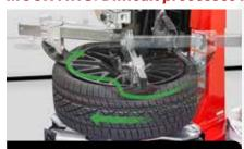
Rising cam action reduces bead stress on top bead mount.
