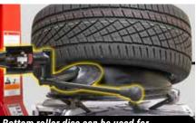
Bottom roller disc can be used for bottom bead reloosening, demounting, or match mounting.
