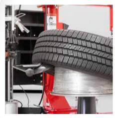
Lower locking disc can demount bottom beads
