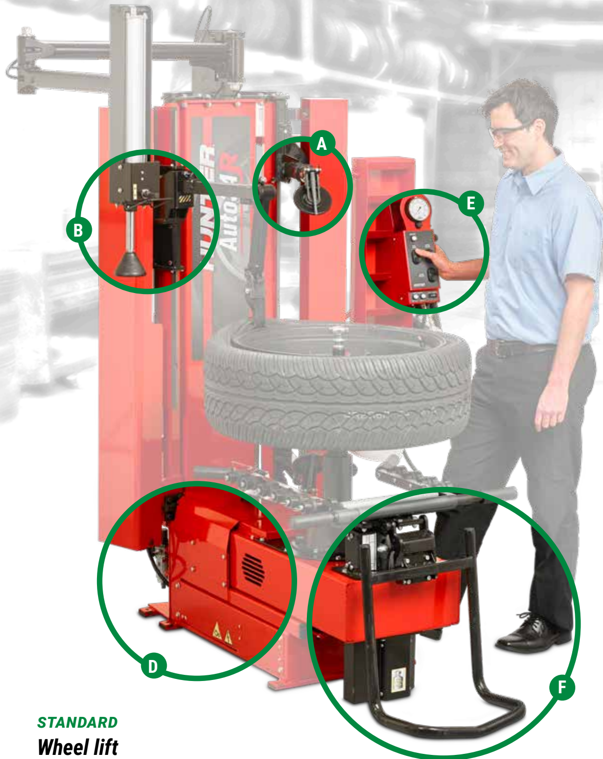
Inflation, rotation and wheel lift operations are controlled by three foot pedals.
