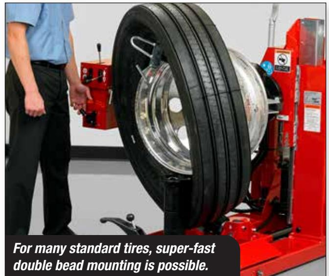
**For many standard tires, super-fast double bead mounting is possible.**
