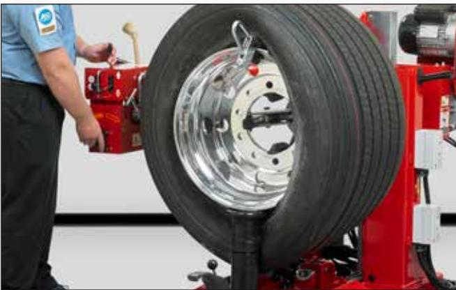
✓ Use standard aluminum or steel rim clamps to assist mounting.
