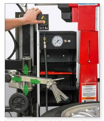
Large tank provides ample volume to seat the toughest tires. Simply set the position, select inflation mode then press the inflation pedal.
