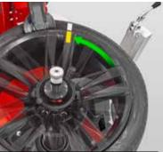
The bead rollers safely hold the tire stationary while the rim is rotated to complete match-mounting.
