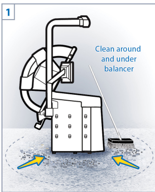
Wheel weights under balancer may cause weight chasing.
