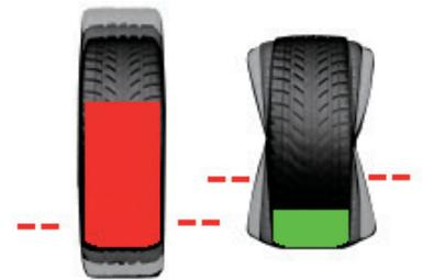
SmartWeight® panel displays wheel balance condition
