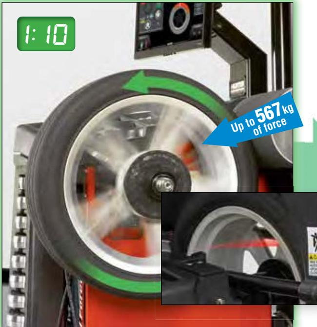
Tire is balanced in less time with Hunter's Road Force® Elite premium diagnostic balancer.
