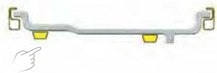
Rim cutaway displays selected weight mode
