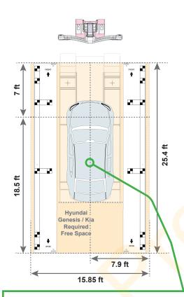
Position vehicle forward or backward as needed to keep mats out of pit for front and rear procedure
