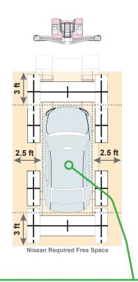
> Position vehicle forward or backward as needed to keep mats out of pit for front and rear procedure COMING SOON
