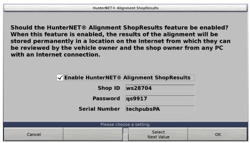
Test the set up by checking HunterNet after performing and printing an alignment. From a different PC, log in to HunterNet at www.hunternetwork.com. Use the same credentials as the aligner. Under the "Alignment ShopResults" tab, users can look at the alignment printout.
