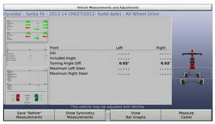
Note that some vehicles in the specification database do not specify a turn reference angle. Toe-out-on-turns can still be measured. When steering to the left and right, the bar graphs are not color-coded and neither is labeled "Steer This Wheel." When steering to the left and right, you must steer the wheels as desired, then press "Ready" to make a snapshot of the measurements.
