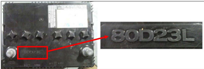
Batteries with JIS (Japanese Industrial Standard) Number
