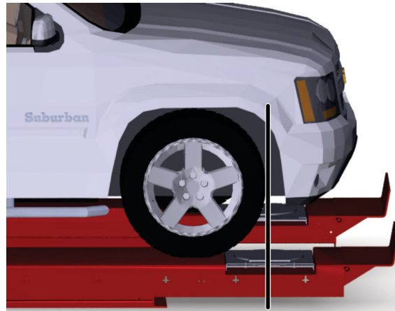
Leading Edge of Tire at Center of Turnplate
