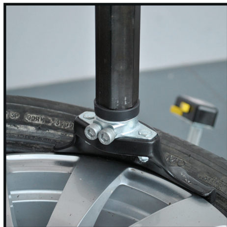
MOUNT HEAD INCORRECTLY PLACED
