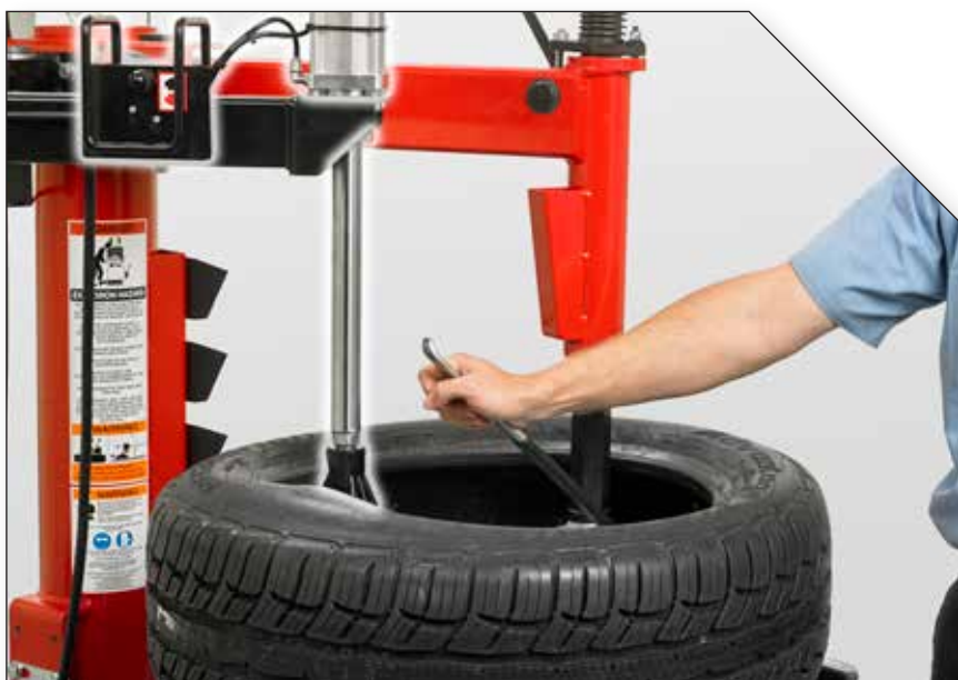
Lifting hook aids the demounting of heavy tires.
