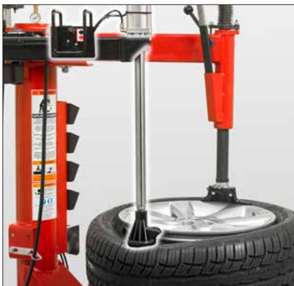
Press arm pushes tire into drop center for mounting and demounting operations
