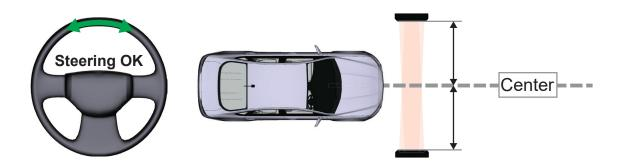
2 Hold steering wheel straight ahead as vehicle approaches towers
