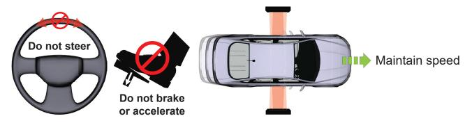
4 Steering movement allowed after vehicle clears sensor towers
