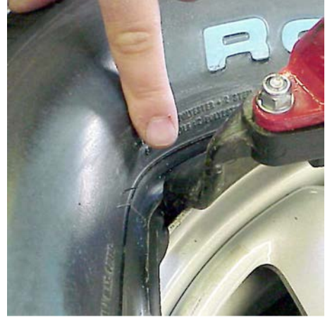
TIRE IS INCORRECTLY PUSHED ON BY MOUNTING HEAD
