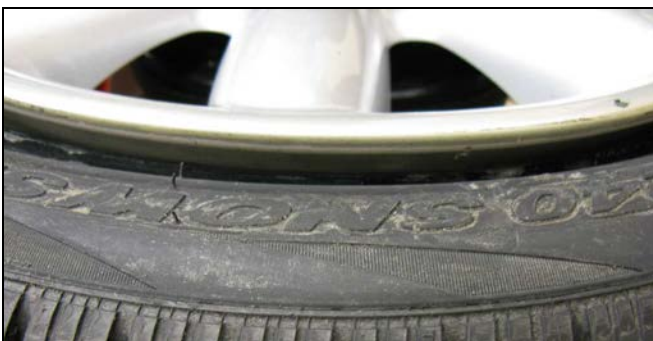
BEAD NOT IN DROP CENTER
