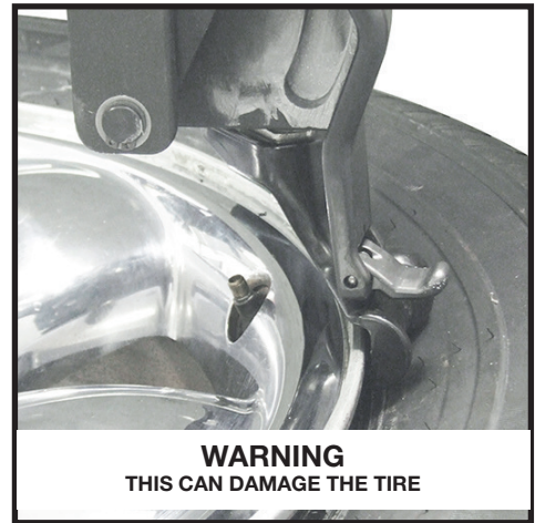
MOUNT HEAD INCORRECTLY PLACED
