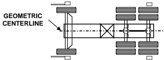
The geometric centerline is (approximately) a line drawn through the midpoints of the front and rear axles.
