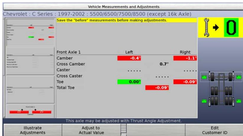
**CAUTION:** Do not confuse the “adjust to zero” and “adjust to actual value” formats. The displays are different to help prevent this. Note especially the large “adjust to zero” icon that appears at the upper right corner when the “adjust to zero” format is used.
