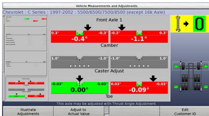
A red bar graph indicates the measurement is out of tolerance. An “X” indicates the measurement is beyond the indicating range of the bar graph in the direction shown. The “X” changes to an arrow indicator when the measurement is adjusted into the indicating range of the bar graph.
