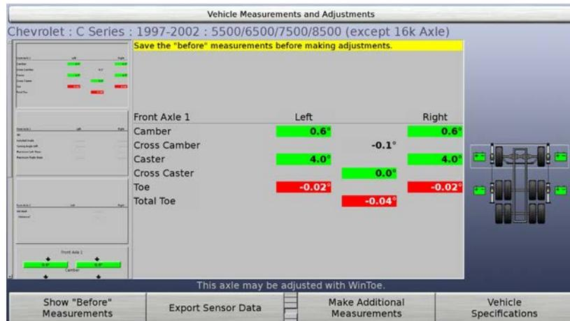
It is displayed by pressing “Measurements and Adjustments.”
