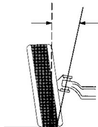
S.A.I. is the angle, as viewed from the front, between the steering axis and the vertical. S.A.I. is measured and displayed in degrees.
