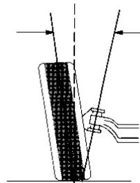
Included angle is the angle, as viewed from the front, between the plane of the wheel and the steering axis. This angle is measured and displayed in degrees. It is computed as the sum of S.A.I. and camber.
