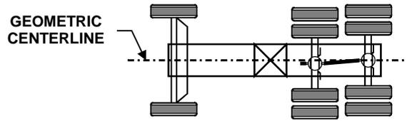
When the geometric centerline does not cross the midpoint of all axles. Negative Tandem Lateral Offset is when the geometric centerline is to the right of the axle midpoint. Positive Tandem Lateral Offset is when the geometric centerline is to the left of the axle midpoint. A tandem lateral offset condition or tread width variation will not affect the accuracy of the system.
