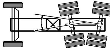
**Thrust Line** is the bisector of total toe angle of the axle. **Tandem Scrub Angle** is the angle formed by the two thrust lines of a tandem.
