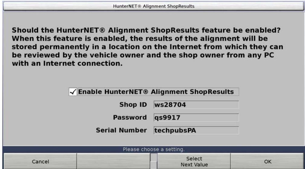
Test the set up by checking HunterNet after performing and printing an alignment. From a different PC, log in to HunterNet at [www.hunternetwork.com](http://www.hunternetwork.com). Use the same credentials as the aligner. Under the "Alignment ShopResults" tab, users can look at the alignment printout.
