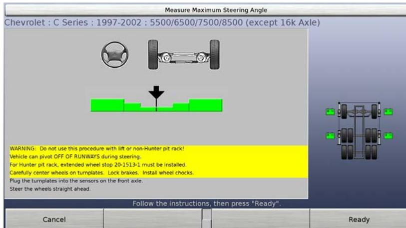
When the "steered straight ahead" measurements have been stored, the display changes to show numbers and prompts you to steer to the left. These numbers show the steering angles of the wheels.
