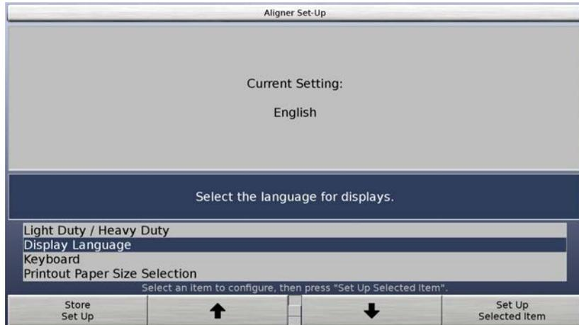
This screen is displayed by pressing “Set Up Aligner” on the start-up screen. It contains a scrolling list of all items that may be set up.
