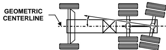
Thrust angle is the angle, as viewed from above, between the geometric centerline and the thrust line of the rear axle. This angle is measured and displayed in degrees.
