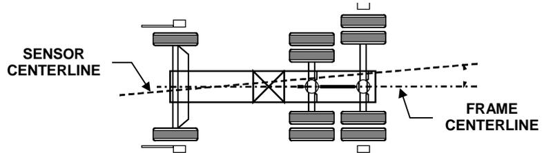
The angle of the frame referenced to the sensor centerline. Frame offset angle is calculated by the aligner when the requested measurements, as shown on the display, are entered into the aligner.
