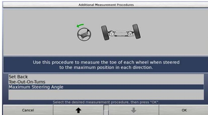
It is displayed by pressing "Make Additional Measurements" on the "Vehicle Measurements and Adjustments" screen.
