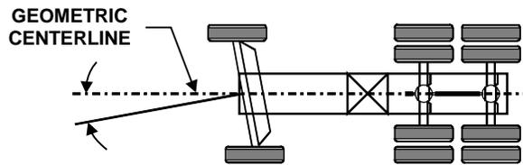
The angle formed by the geometric centerline and a line drawn perpendicular to the front axle. Set back is positive when the right wheel is behind the left wheel. Set back is negative when the left wheel is behind the right wheel. A set back condition will not affect the accuracy of the system.
