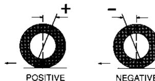
Caster is the angle, as viewed from the side, between the steering axis and the vertical. This angle is measured and displayed in degrees. Caster is positive when the top of the steering axis is tilted rearward and is negative when the top of the steering axis is tilted forward.
