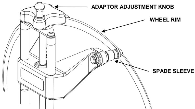
Test the security of the installation by tugging on the wheel adaptor.
