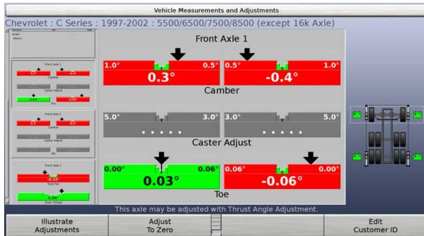
When using the “adjust to zero” format, the number below the bar graph is the difference between the measured value and the specification. You can toggle between the “adjust to zero” and “adjust to actual value” formats by pressing “Adjust to Zero” and “Adjust to Actual Value.”
