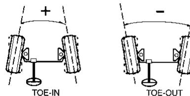
Total toe is the angle, as viewed from above, between the planes of the wheels on an axle. Total toe is measured in degrees but may be displayed in degrees, inches or millimeters. Toe is positive (toed-in) when the front edges of the wheels are closer to the each other than the rear edges of the wheels. Toe is negative (toed-out) when the rear edges of the wheels are closer to the each other than the front edges of the wheels.
