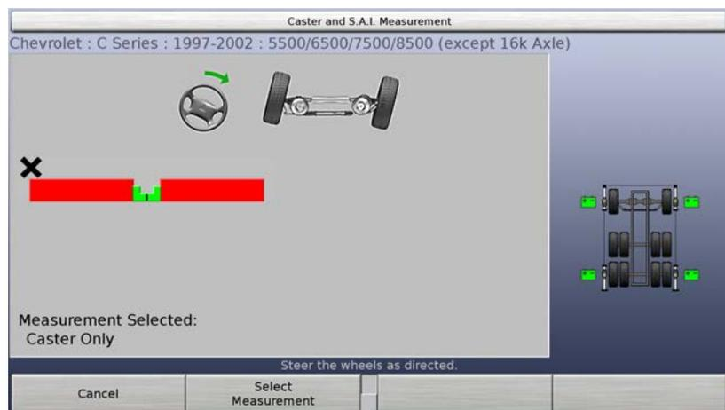
Steer the wheels to the right. When one of the bar graphs is centered, hold the steering wheel steady and allow the system to take a “snapshot” of the measurements. The bar graph disappears when the measurements are stored. Then slowly steer the other wheel until its bar graph is centered, and again hold the steering wheel steady to allow the system to take a “snapshot” of the measurements.
