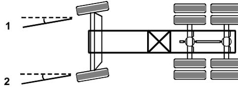
Turning angle is the difference between the toe angles of the front wheels when one of the wheels is steered to a specified turn angle. The two wheels are not parallel to each other due to total toe and to “Ackerman steering.” Ideally, all four wheels steer about the same point.
