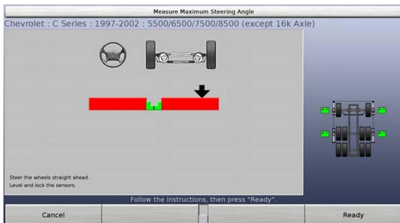
Steer the wheels straight ahead until the bar graph is centered. Then hold the steering wheel steady and allow the system to take a “snapshot” of the measurements.
