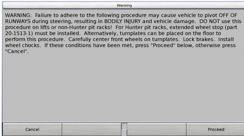
It is displayed when selected on the "Additional Measurement Procedures" screen.
