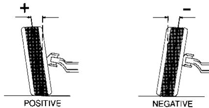
Camber is the angle, as viewed from the front, between the plane of the wheel and the vertical. This angle is measured and displayed in degrees. Camber is positive when the wheel is tilted outward at the top and is negative when the wheel is tilted inward at the top.
