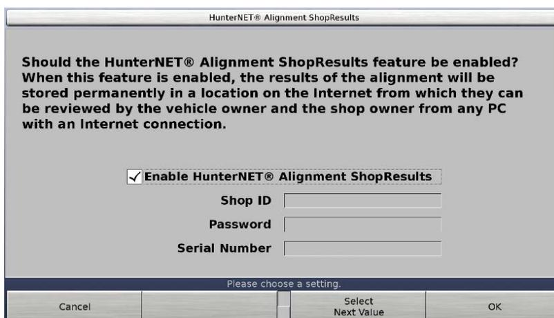
**NOTE:** A separate PC with internet connection is required to perform initial HunterNet account setup and to view the ShopResults generated by the alignments performed. There is no web browsing capability built into ProAlign.
