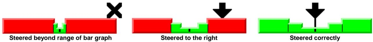
NOTE: Steer the wheels using only the steering wheel. Do NOT manually push or pull the wheels to steer them.
