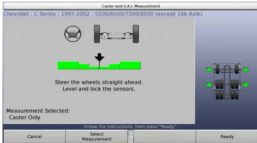
Depress the brake pedal and steer the wheels straight ahead until the bar graph is centered. Level and lock the sensors, then press “Ready” and allow the system to take a “snapshot” of the measurements.
