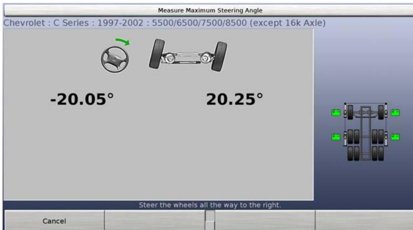
Steer the wheels to the right as far as they will go. Press “Ready” and allow the system to take a “snapshot” of the measurements.
