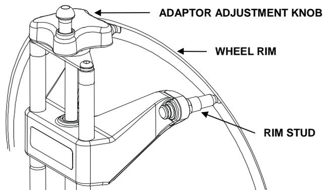
Test the security of the installation by tugging on the wheel adaptor.
