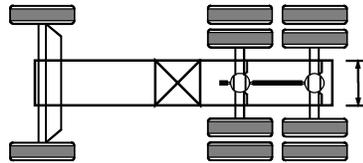
The distance between the reference axle adjustment points. This distance may be measured and entered into the aligner before adjusting thrust angle to allow the aligner to calculate how much the axle must be moved at the adjustment point.
