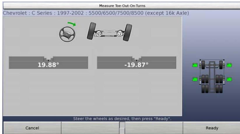
Steer the wheels to the right to center the bar graph labeled “Steer This Wheel.” Hold the steering wheel steady and allow the system to take a “snapshot” of the measurements. The example shown above uses the outside wheel as the reference.
