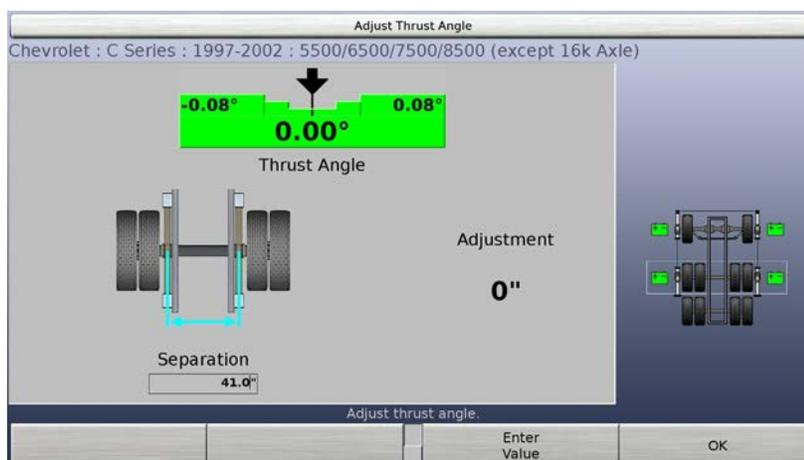
Measure the distance between the reference axle adjustment points. Type in this separation distance, then press “OK” to accept the separation distance, or press “Enter Value” to enter a different value.
