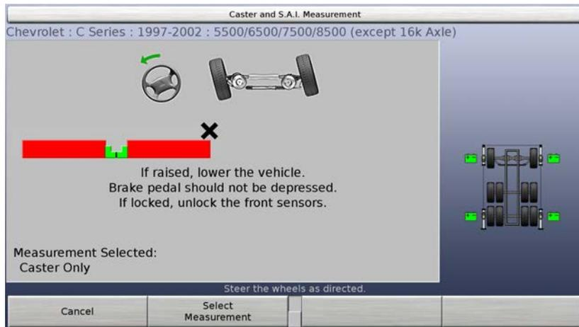
Steer the wheels to the left. Once the bar graph turns green, it will take a snapshot of the position and the bar graph will disappear.
