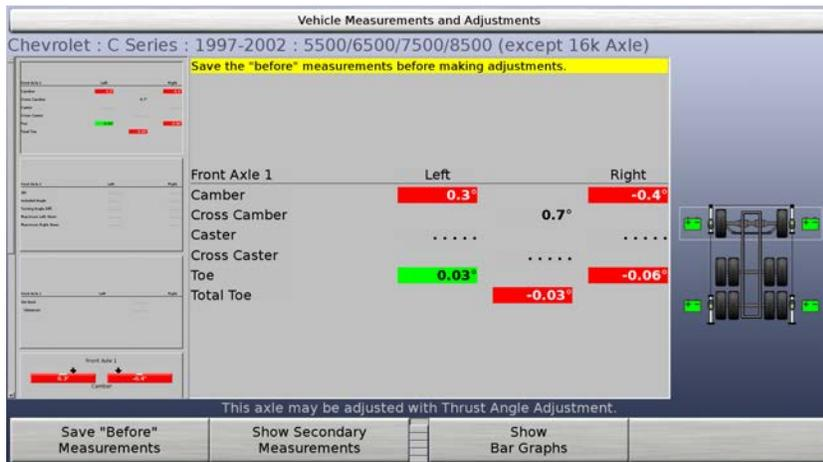
When shown in the “adjust to zero” format, this display is normally used to make adjustments to the vehicle. You can toggle between the “adjust to zero” and “adjust to actual value” formats by pressing “Adjust to Zero” and “Adjust to Actual Value.”
