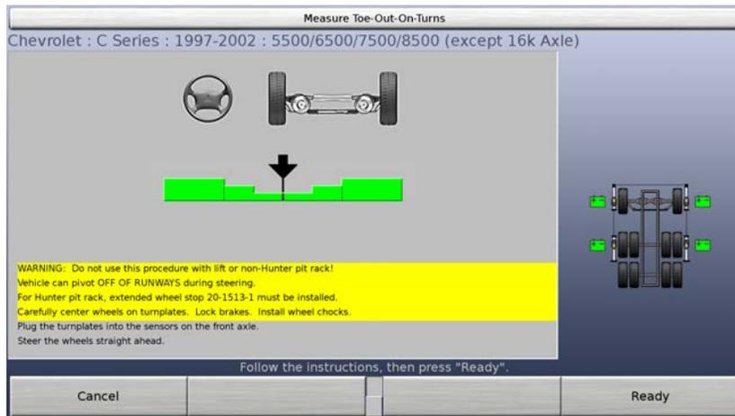
When the “steered straight ahead” measurements have been stored, the display changes to show two bar graphs and prompts to steer to the left.
