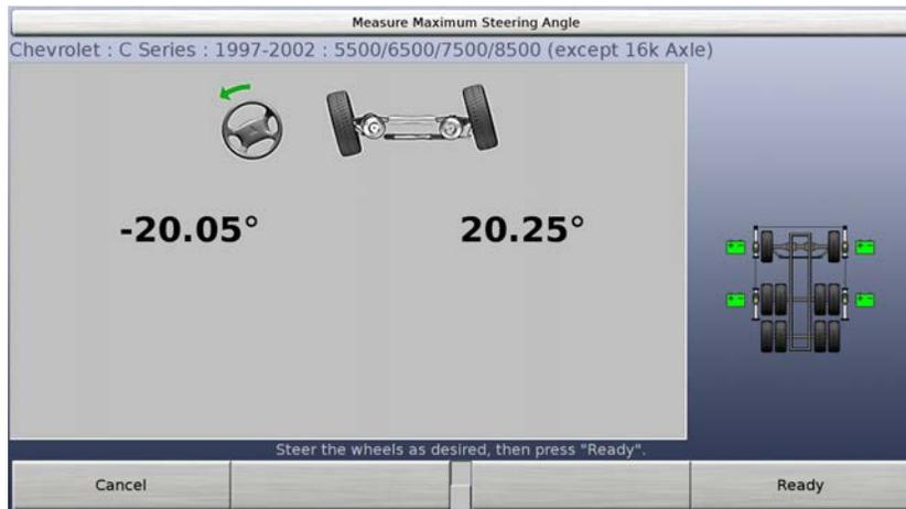
Steer the wheels to the left as far as they will go. Press “Ready” and allow the system to take a “snapshot” of the measurements.
