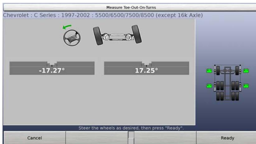
The left bar graph shows the steering of the left wheel while the right bar graph shows the steering of the right wheel. One bar graph will be color-coded and will be labeled “Steer This Wheel.” The other bar graph will be gray. Each bar graph shows the steering angle of the corresponding wheel if specs are available.
