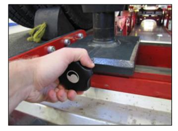
After the load on the cylinders is removed, turn the control valve handle downwards to lower the rams completely while keeping release knob open.
