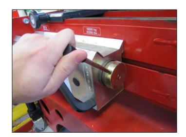
Turn the control valve further upwards to the second stage to begin lifting vehicle.
