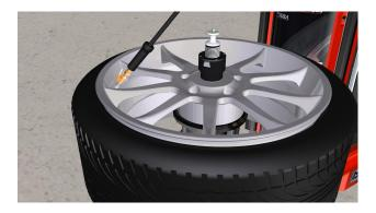
2. The bottom right interface tab shows inflation controls. Touch the left and right arrows above the pressure gauge to adjust the target air pressure.
