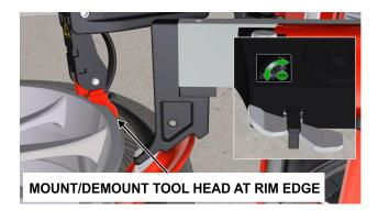
2. The lower roller will raise with the mount/demount tool head with bead hook. The wheel assembly will then rotate clockwise as the bottom bead is fully demounted. The wheel assembly will then rotate clockwise as the top bead is fully demounted.
