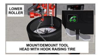
1. Verify the TPMS is in the four o'clock position. If not, press and hold the right "GO" side of the pedal and let the tire changer finish automatic positioning.
