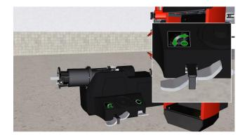
3. With top of the spindle in the rim center hole, press and hold down the right side of the pedal to raise the wheel assembly. Release the pedal when the wheel assembly reaches operating position.
