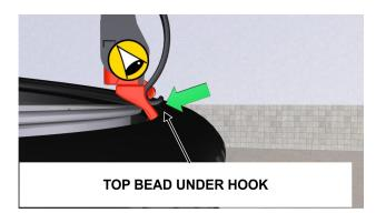
2. To use press arms, manually rotate both arms fully counter clockwise. The press arms and upper roller will lower automatically at correct part of mounting process.
