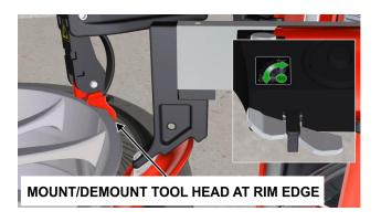
2. The lower roller will raise with the mount/demount tool head with bead hook. The wheel assembly will then rotate clockwise as the bottom bead is fully demounted. The wheel assembly will then rotate clockwise as the top bead is fully demounted.
