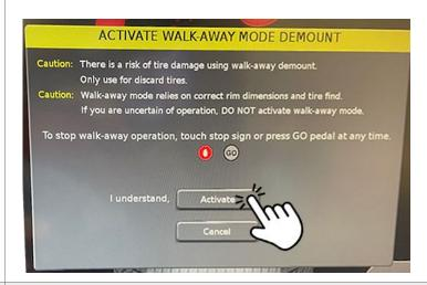
5. If the operator selects "Activate" the tire changer will begin autonomous demounting of the tire. Touching the screen (stop sign) or any control (joystick, pedal, or estop) will immediately halt walkway and it will need to be re-enabled by performing a new complete "operator present" tire change.
