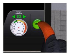
After beads have been seated, disconnect inflation hose and reinstall valve stem core previously removed. Re-connect the inflation hose and inflate tire to the specified target pressure. Disconnect the inflation hose.
