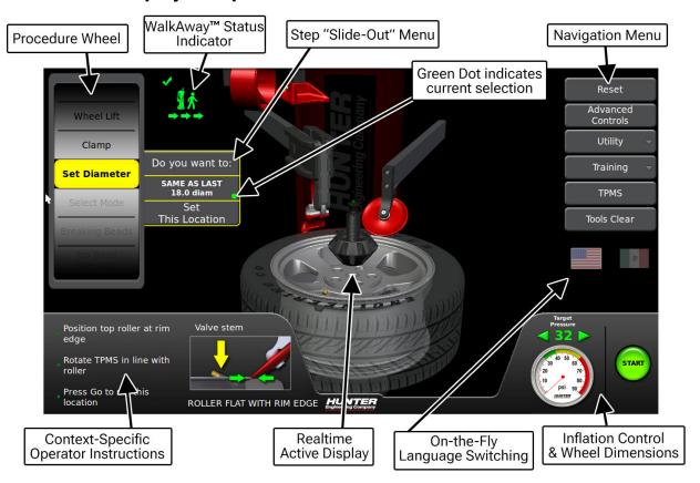
A procedure wheel is located on the left side of the screen. Steps can be skipped and accessed by rolling the wheel up or down and touching the desired selection. In most cases, touching a selection initiates a "slide-out" menu providing additional functions.
