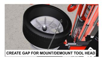
3. Using a clenched fist, push down on the sidewall of the tire while pressing and holding the right "GO" side of the pedal.
