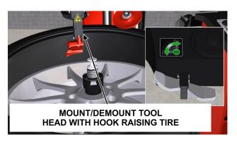
2. The lower roller will raise with the mount/demount tool head with bead hook. The wheel assembly will then rotate clockwise as the bottom bead is fully demounted.
