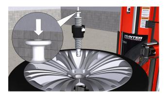
2. When the clamp is properly inserted, the button on the top of the clamp will spring up, showing the green band. If the green band is not visible, re-seat the clamp. *Do not proceed unless the green band is visible.*
