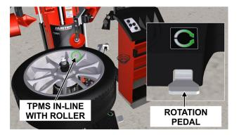
2. The TPMS sensor should be directly in-line with the upper roller.
