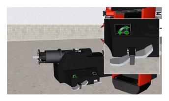
3. With top of the spindle in the rim center hole, press and hold down the right side of the pedal to raise the wheel assembly. Release the pedal when the wheel assembly reaches operating position.
