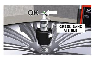
3. Press and release the right "GO" side of the pedal to fully seat the clamp and secure the wheel.
